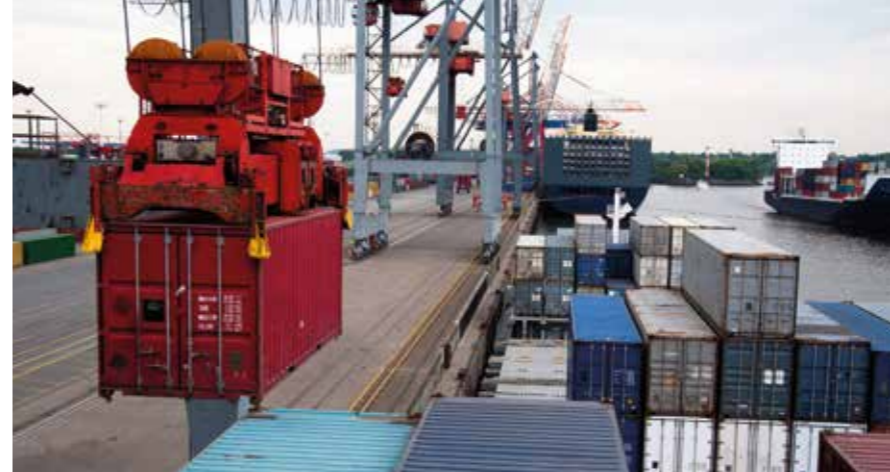
Rail-bound mobile harbour crane handling containers.
