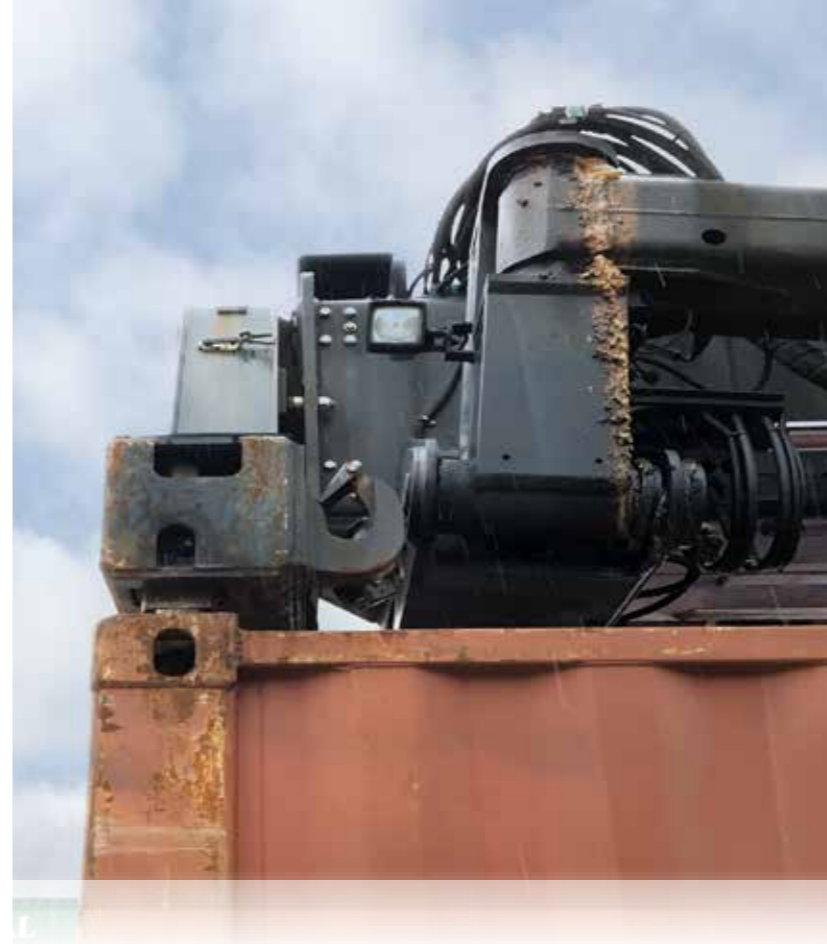
The cameras are mounted in such a way as to provide an optimum view onto the twistlocks.
