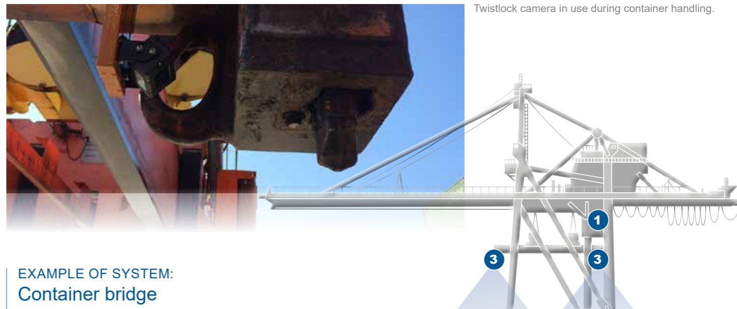
Twistlock camera in use during container handling.
